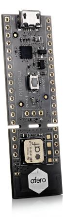
Flexible Form Factor Use Modulo-1 standalone, or as a tool to enhance your Arduino project. Modulo-1 attaches to a compatible Arduino<sup>®</sup> board (such as Uno) via the Afero Plinto<sup>™</sup> shield, or to a Teensy development board directly.
